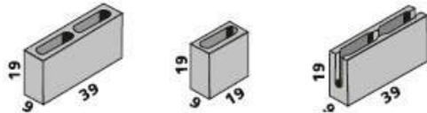
**BLOCO CLASSE C -  $f_{bk} \geq 3,0 \text{ MPa}$**
